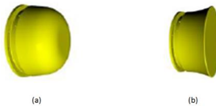
Figure10: Kinds of Cap (a) Convergent Cap (b) Divergent Cap [8]
