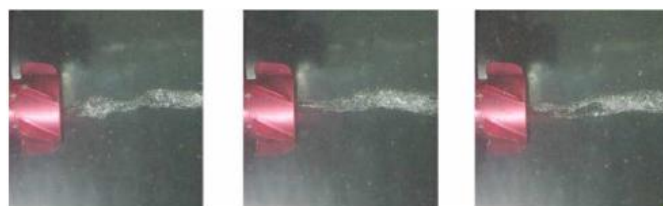
Figure 6: Vortex on PBCF with divergent hub type [1]
