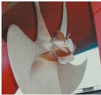
Figure.3 Propeller Boss Cap Fins [13]
